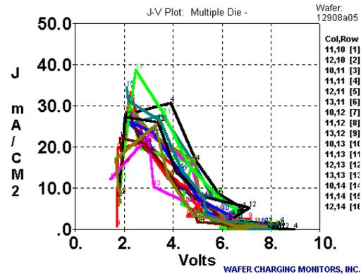
Figure 8. CHARM-2 positive J-V plots in the plasma oxide deposition tool.
