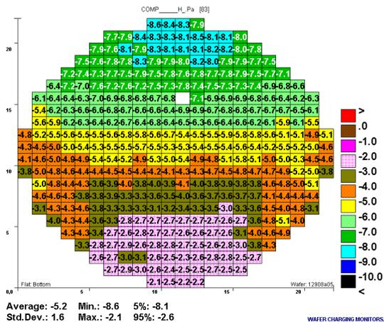
Figure 11. CHARM-2 map of negative potentials in the plasma oxide deposition tool.
