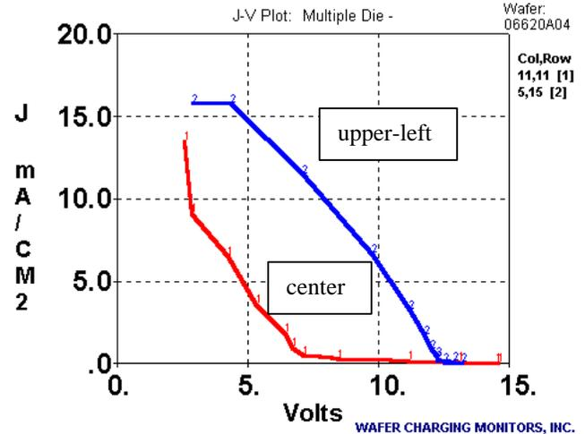
Figure 3. Positive current density in the center and upper-left of the wafer.
