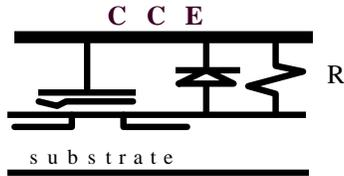
Figure 9. CHARM-2 unipolar positive charge-flux sensor: CCE = charge collection electrode; R = current sensing resistor. (The charge-flux sensors used to obtain the J-V plots in Figure 8 do not use a diode.)
