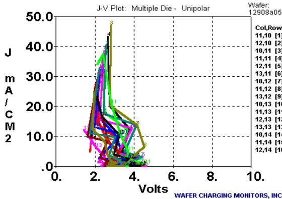
Figure 10. CHARM-2 positive J-V plots obtained in the oxide deposition tool with the unipolar charge-flux sensors.
