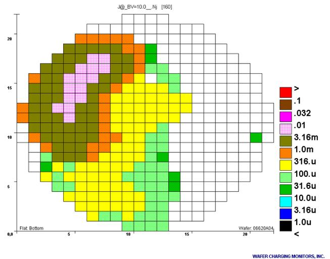
Figure 4. DamageMap™ of net positive current density in A/cm<sup>2</sup> (at  $BV_{ox} = 10$  V) reaching the surface of the wafer.
