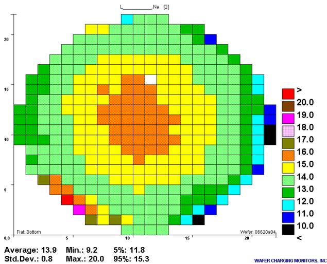
Figure 2. ChargeMap® of surface-substrate potentials in oxide deposition.
