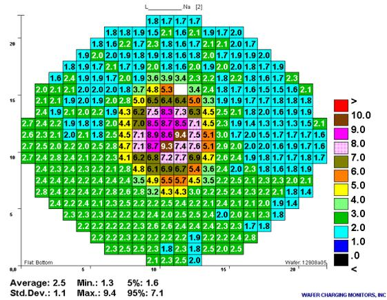
Figure 7. CHARM-2 map of positive potentials in the plasma oxide deposition tool.
