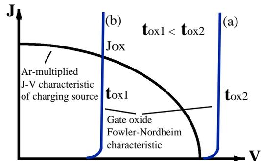
**Figure 1.** Oxide damage prediction: **(a)** F-N plot does not intersect A.R.-multiplied JV plot: damage is not possible; **(b)** F-N plot intersects A.R.-multiplied JV plot: damage is likely. (Note: A.R. = Antenna Ratio.)
