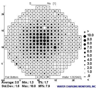
Figure 4a. Positive potentials recorded in a plasma tool #1 with a bare CHARM®-2 wafer containing scribe-lane process control structures.
