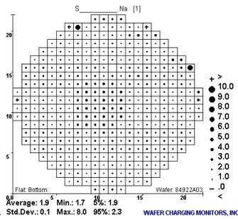
Figure 4b. Positive potentials recorded in a plasma tool #1 with a bare CHARM®-2 wafer without scribe-lane process control structures.
