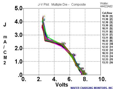
Figure 3b. Positive J-V plots recorded in the center of a bare CHARM<sup>®</sup>-2 wafer with small charge collection area connected to the substrate. Peak potentials of ~ 8 V were recorded. (The vertical asymptote at ~ 2.4 V is an artifact of the data conversion procedure, and should be ignored.)
