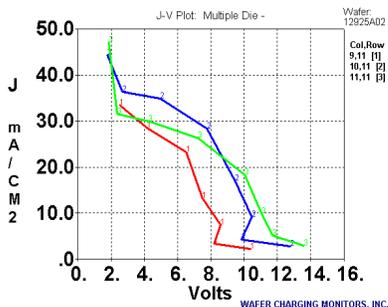
Figure 2. Positive current density caused by “electron shading” in HDP oxide etcher. Curve “1” corresponds to 0.6 um holes; curve “2” corresponds to 0.3 um holes; curve “3” corresponds to 0.15 um holes.
