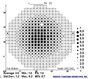
Figure 5b. Positive potentials recorded in a plasma tool #2 with a bare CHARM®-2 wafer without scribe-lane process control structures.
