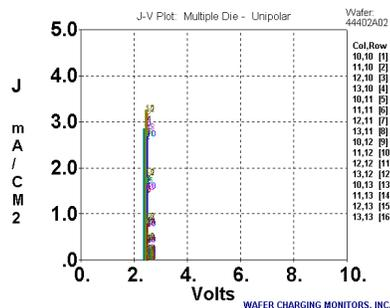
Figure 3a. Positive J-V plots recorded in the center of a bare CHARM<sup>®</sup>-2 wafer with large charge collection area connected to the substrate. The vertical line at ~ 2.3 V indicates that the charge-flux sensors did not respond, i. e., positive potentials were less than ~ 2.3 V.
