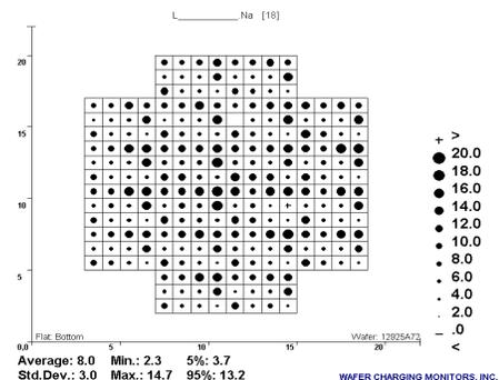
Figure 1. Positive potentials caused by “electron shading” in HDP oxide etcher.
