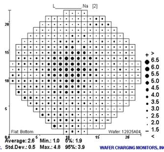
Figure 5a. Positive potentials recorded in a plasma tool #2 with a bare CHARM®-2 wafer containing scribe-lane process control structures.
