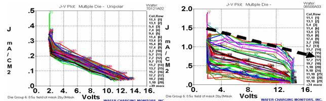
Figure 4. (a) uniform plasma produces uniform positive charging over entire wafer in 0.5 um holes (in 1.2 um resist); (b) non-uniform plasma produces non-uniform, and greatly enhanced, positive charging (note J scale change).
