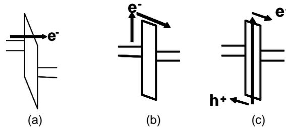
Figure 1. (a) Charge transport at very high electric field (tunneling); (b) UV-enabled charge transport ( $3.2 \text{ eV} < E < 9 \text{ eV}$ ); (c) UV-enabled charge transport ( $E > 9 \text{ eV}$ ).
