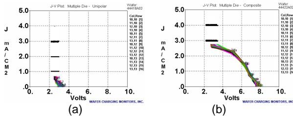
Figure 5. Positive charging caused by identical antennas connected to transistor gates increases (J-V plots move to higher voltages) when the size of antennas connected to wafer substrate decreases: (a) large antenna; (b) small antenna.
