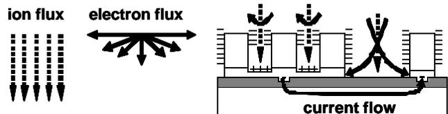
Figure 3. The anisotropic ion flux and isotropic electron flux in etching plasmas cause positive charging at the bottom of narrow trenches, and negative charging at the bottom of wide trenches.
