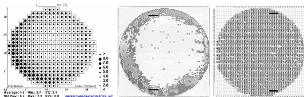
Figure 2. (a) positive potentials during via etch, (b) die around periphery fail margin tests (black = fail), (c) programmed die fail margin tests after forming gas anneal.
