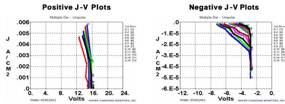
Figure 6(a). High positive charging is observed during a high current implant when PFS is turned OFF.
