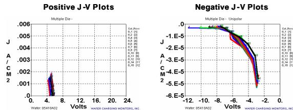
Figure 6(b). Positive charging is reduced (positive J-V plots move to lower voltages) and negative charging is increased (negative J-V plots move to higher voltages) during the same implant when PFS is turned ON.
