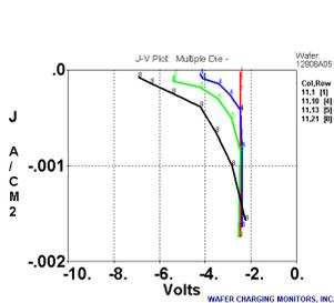
Fig. 13. Oxide deposition: Negative J-V: top to bottom.
