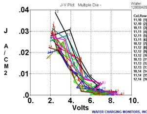
Fig. 11. Oxide deposition: Positive J-V from wafer center.
