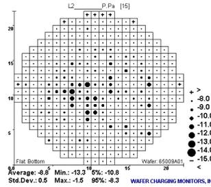
Fig. 6. Unstable plasma: Negative potentials obtained with a single potential sensor.
