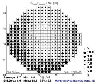
Fig. 9. Oxide deposition: CHARM-2 UV response.
