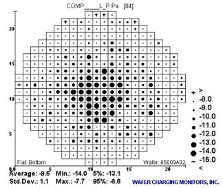
Figure 7. Unstable plasma: Negative potentials obtained with multiple potential sensors.
