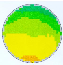
Fig. 14. Oxide deposition: SPM map.
