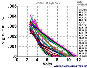
Fig. 4. HDP: Positive J-V from wafer periphery<sup>3</sup>.
