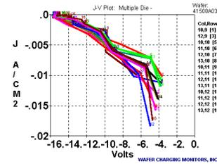
Fig. 5. HDP: Negative J-V from wafer center.
