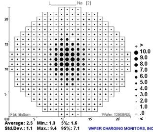
Fig. 10. Oxide deposition: CHARM-2 UV Positive potentials.
