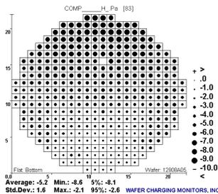
Fig. 12. Oxide deposition: CHARM-2 Negative potentials.
